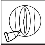
Apply adhesive to the area around the hole on the inside of the FlexiTank itself.
