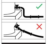
When elevating your FlexiTank on a stand, install your in-line filter away from the FlexiTank tap to prevent tension against the FlexiTank.
