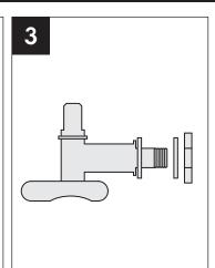
To fit the tap into the Tap Hole first take the tap, remove the nut and ONE washer from the tap thread.
