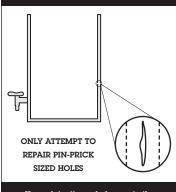
Upon detecting a hole empty the FlexiTank immediately. Disconnect the FlexiTank. Dry the FlexiTank using cloth etc.
