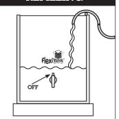
When refilling the FlexiTank turn the tap off. Refill and leave for 60 mins before turning back on. This prevents sediment being pulled through pipes whilst refilling.
