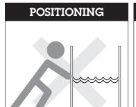
Never attempt to drag or otherwise move a FlexiTank when in use, regardless of the fill level. Get your FlexiTank correctly positioned before filling.
