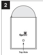
Undo the FlexiTank zip and open the FlexiTank tank up - logo outside. Locate the Tap Hole towards the base.
