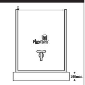
If using with a gravity fed system always raise your FlexiTank to a minimum of 150mm / 6" above the highest module.
