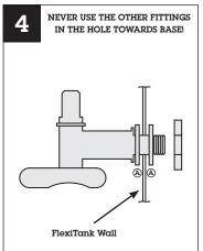
Push the tap through the FlexiTank, fitting the rubber washers as shown (A)
