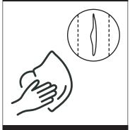
Ensure the inside of the FlexiTank is clean and dry - YOU WILL BE APPLYING YOUR PATCH TO THE INSIDE SURFACE.
