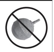
Do not place an air stone in the FlexiTank as this can raise pH levels of the nutrient solution. A water pump may be used to agitate the solution but is not necessary.
